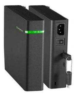
Network-attached storage (NAS) refers to a data storage server that is connected to a computer network. NAS systems allow multiple devices to access the same storage over a variety of network infrastructure technologies. Some examples of Ciphertex NAS products include portable NAS servers and rackmount NAS servers.
